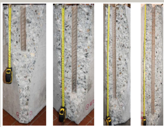
Fig. 10b - Influence of anchorage length on bond strength
